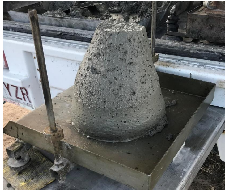
Figure 2 – Great White HRM™ concrete sample, showing enhanced form retention
