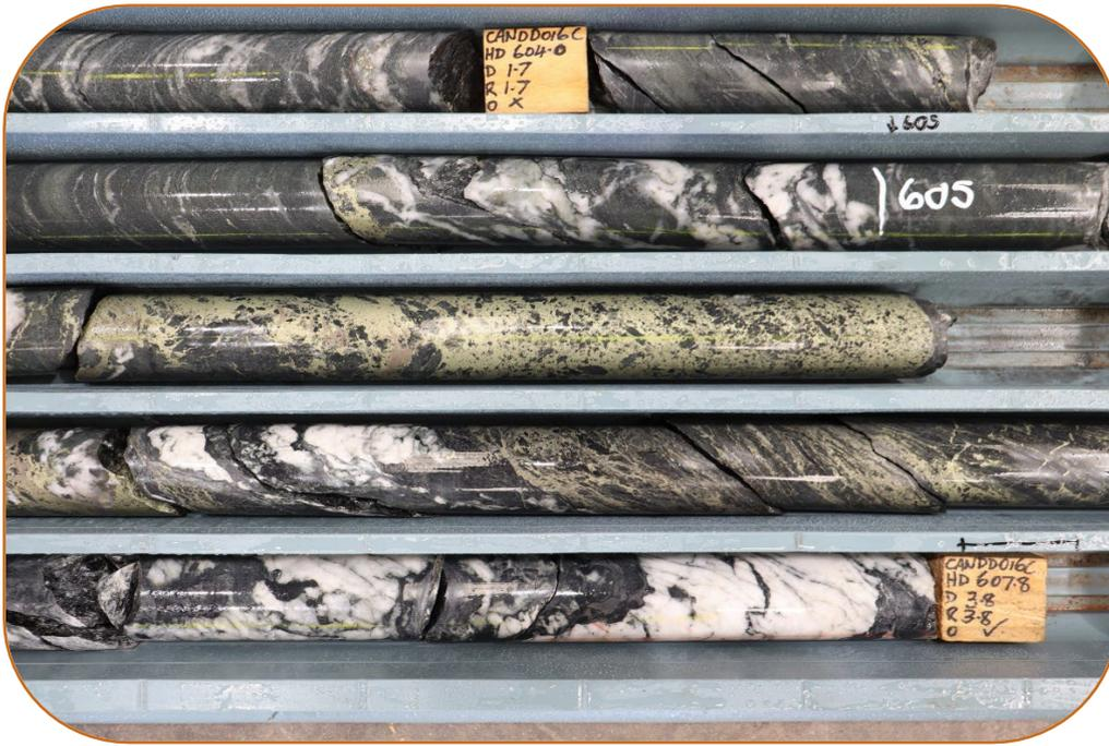
**Figure 1b** – Chalcopyrite occurring as semi massive, vein and stringer textures (CANDD016C)
