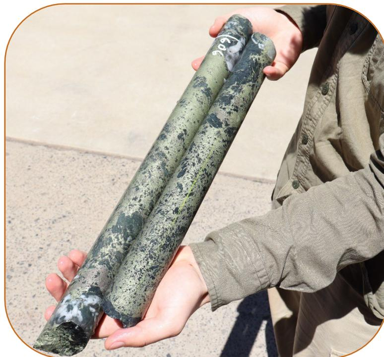
**Figure 1a** – Semi massive chalcopyrite mineralisation in drill core from CANDD016C
