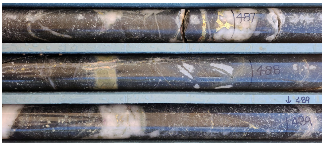
Figure 1. Mineralised drill core from 22BRD0014 between 486.5m and 489.0m down-hole depth. Note multiple phases of quartz-chalcopyrite+/-anhydrite+/-K-feldspar veining cutting weakly porphyritic volcanic-sediments/fragmental rocks. Visually estimated chalcopyrite abundance ~1% by volume. HQ3 core (63.5mm diameter).*
