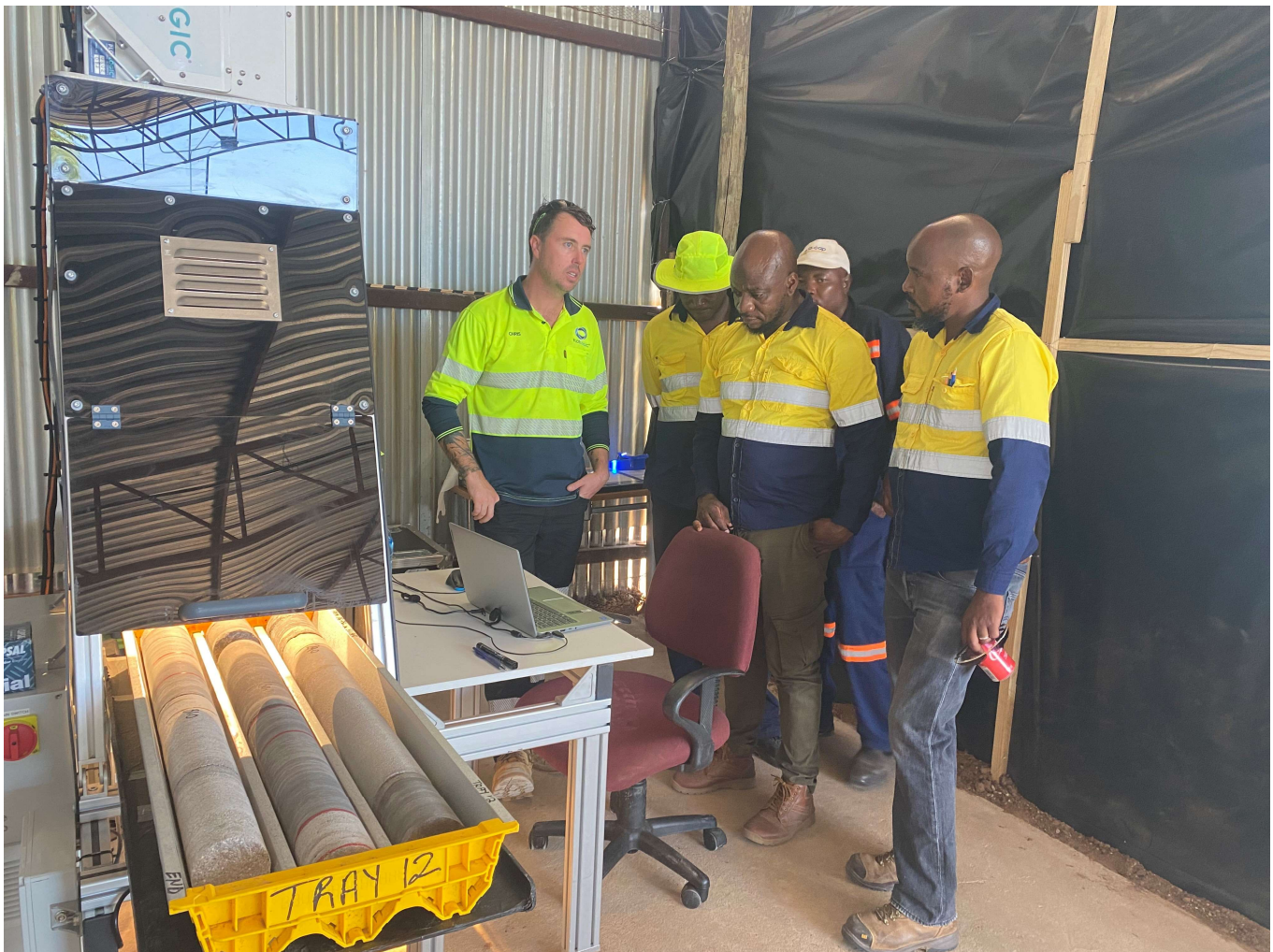
Figure 2 Hyperspectral Scanner scanning PQ at A-Cap core facility in Gijwane.
