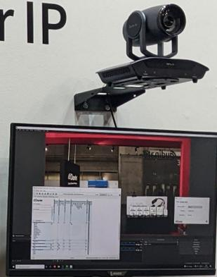
A monitor displaying the Dante AV control interface, which includes a video feed and various control panels for audio and video management.
