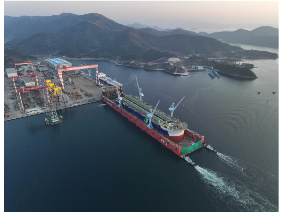
Barossa FPSO entering floating-dock for assembly
