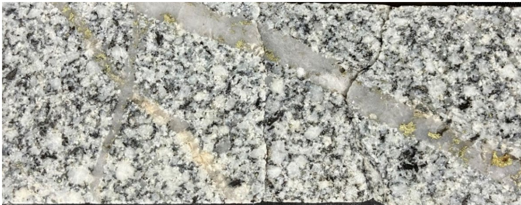
Figure 1 Copper sulphides in mineralised granodiorite. Hole 23BRD0016 at 123.5m. Within a 2m interval of 63.5mm diameter core which assayed 0.31% Cu.
