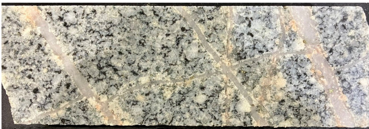
Figure 4 Mineralised and altered porphyritic granodiorite at 76.5m down-hole depth in 23BRD0016. From within a 2m sample of 63.5mm diameter core which assayed 0.31% Cu.
