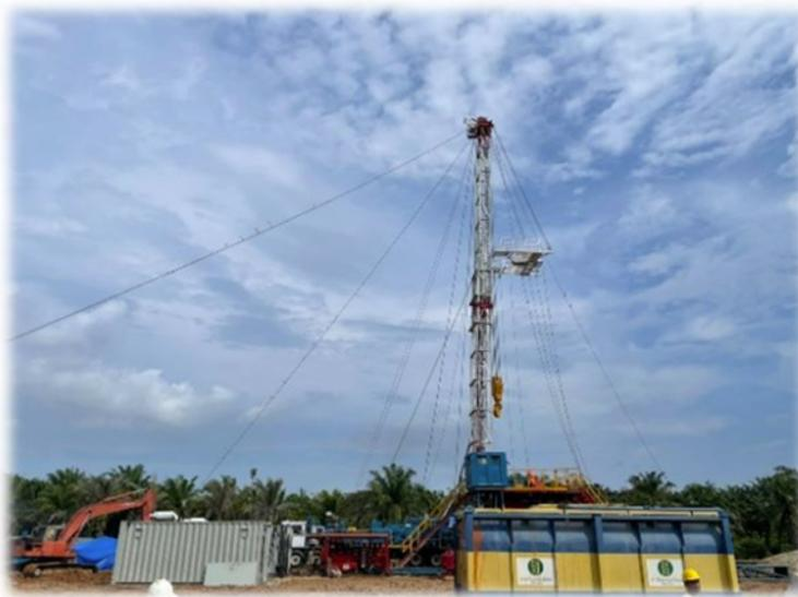
BA-01 is planned as a **vertical exploration well approximately 2800ft in depth** and will be suspended if successful. The well aims to test the presence of hydrocarbons in the BA prospect, primarily targeting the Miocene-age Telisa Formation sandstone reservoir located at a depth of 900ft. A secondary target is the Menggala Formation, expected at approximately 2500ft. **Both targets are producing reservoirs in the Central Sumatra Basin.**
