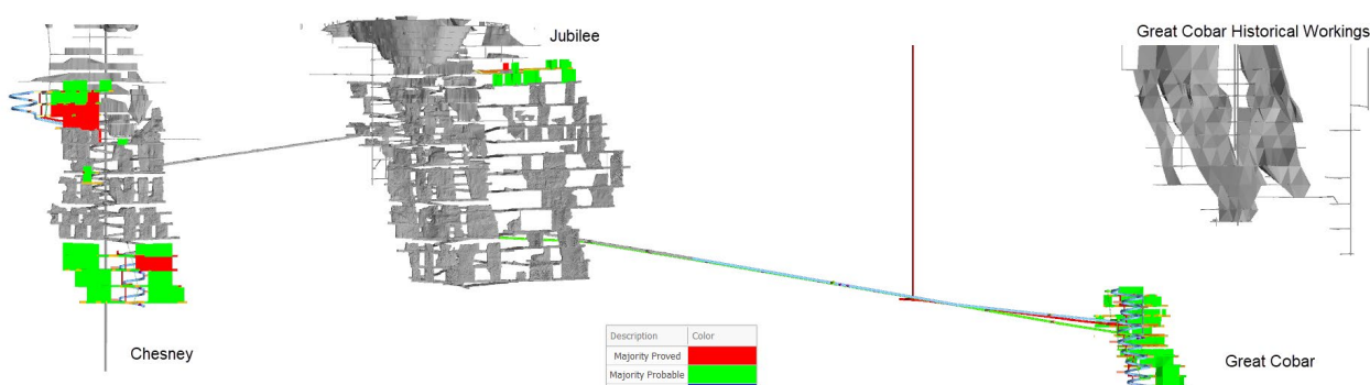
Figure 7. Long section facing west of the Peak North Mine showing Proved (red) and Probable (green) Ore Reserve classifications.
