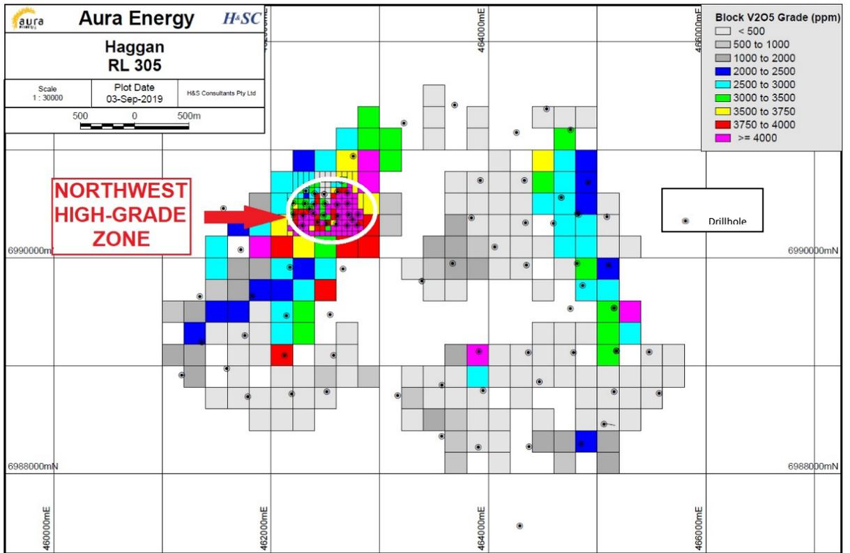
Figure 5: Horizontal section (plan view) of the Häggån Resource at approximately 45 metres below surface
