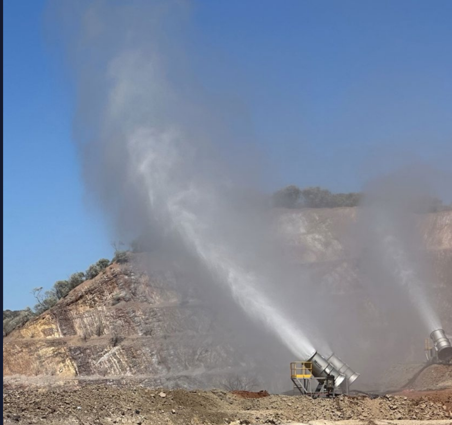
Evaporators at Capricorn Copper
