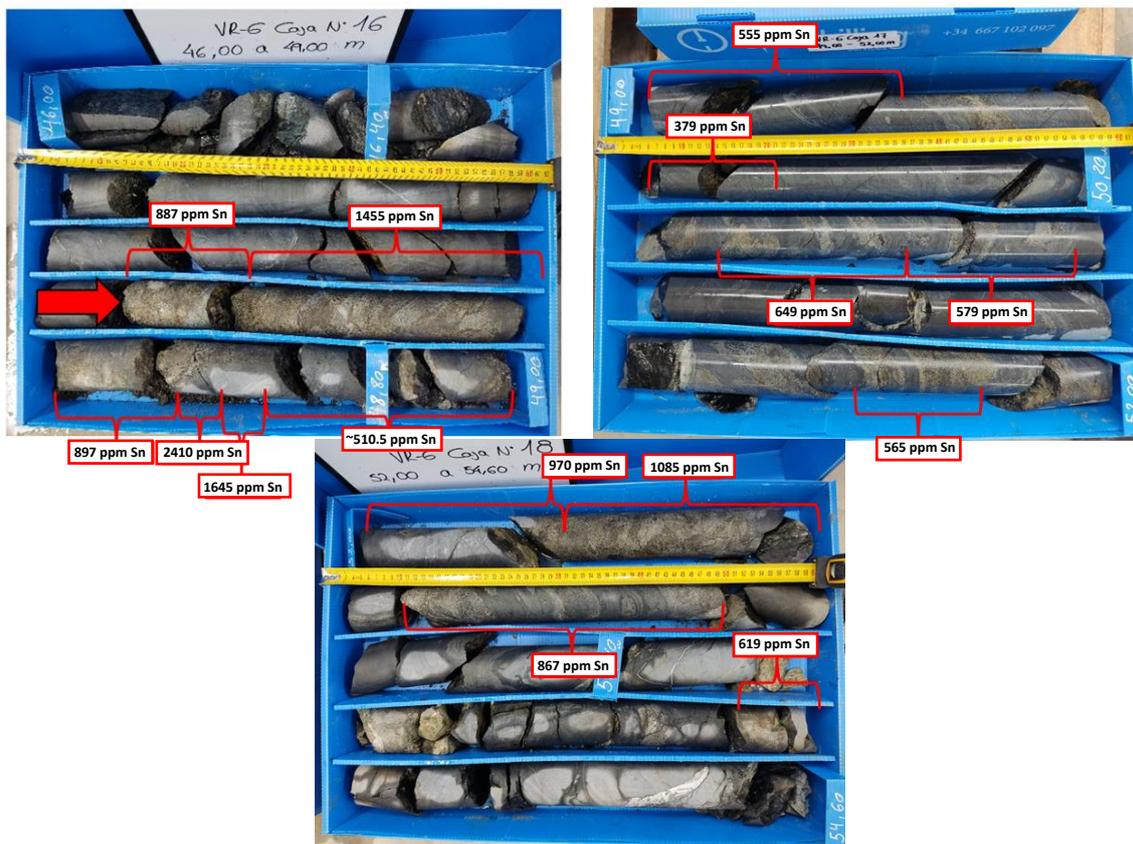
Figure 3: Hole VR-06 core trays from 46m to 54.60m. Contact between fresh and altered metasedimentary rocks marked by the red arrow. Tin content in several sections of the altered metasedimentary rock.
