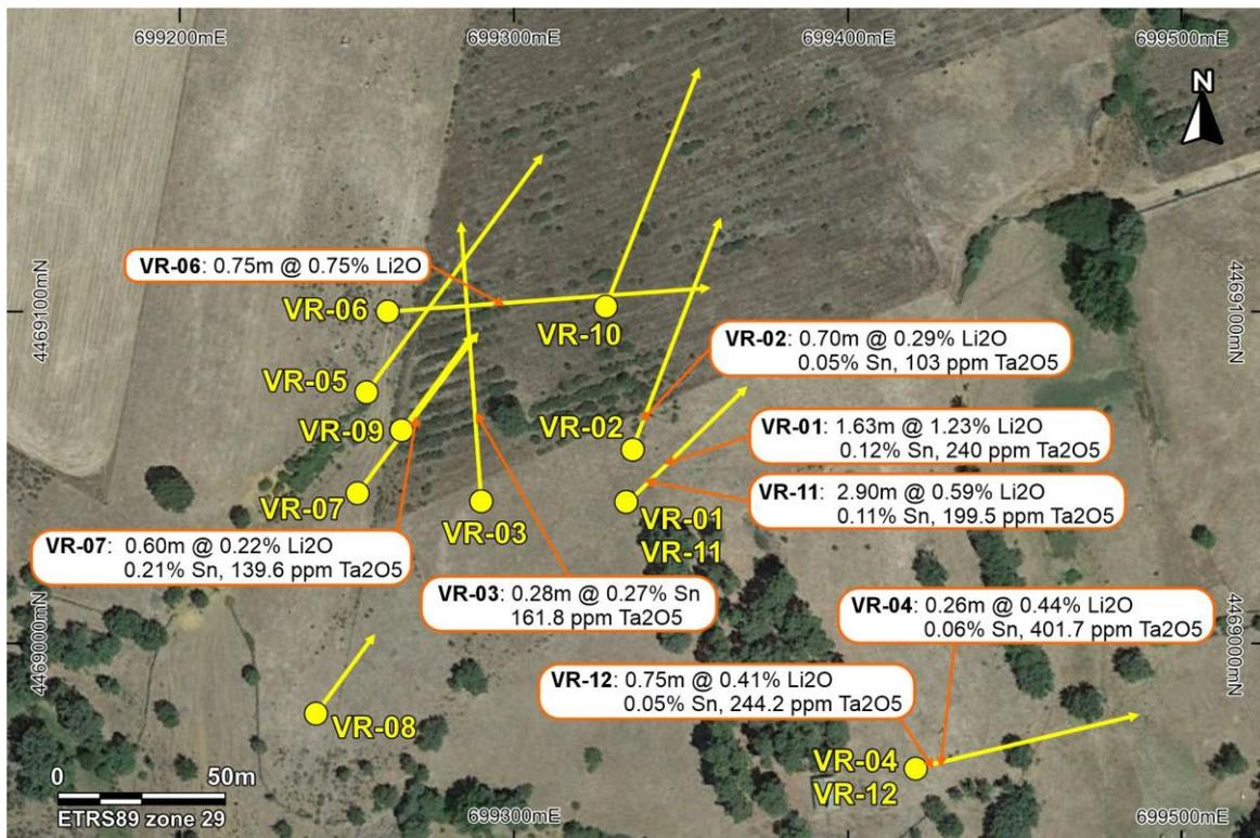
Figure 2: Villasrubias drill hole location showing significant intercepts.
