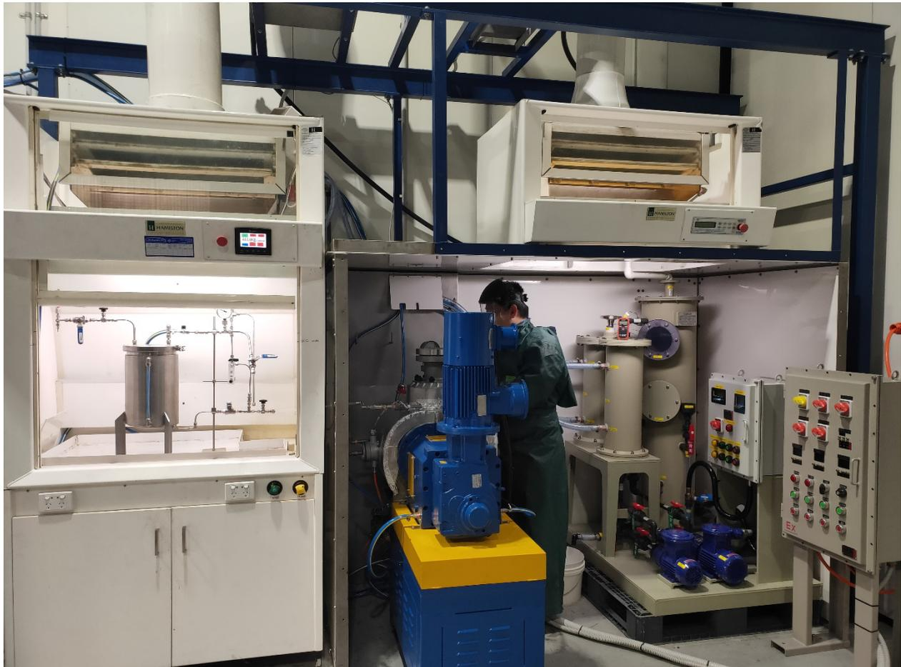
**Figure 1: Bath pilot batch reactor (centre) installed at ALCORE Technology Centre**
