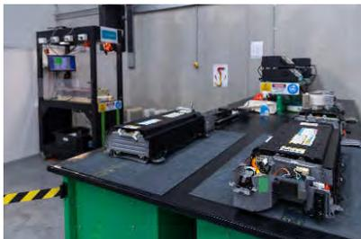
Infinitev battery testing station
