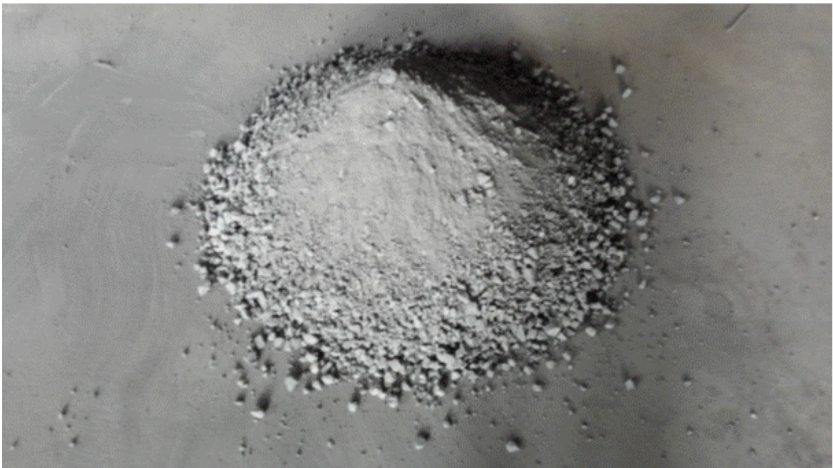
Figure 7-2. Core sample - HPGR product for mineral processing tests. Source: Magang (2018).
