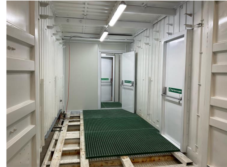
Wellhouse Container with bunding under fabrication
