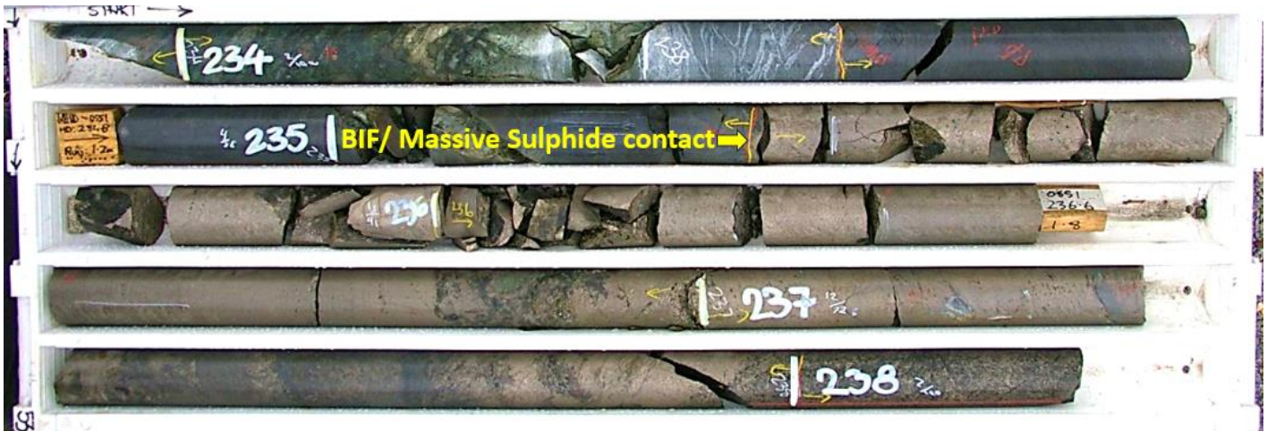
FIGURE 3: HISTORICAL CORE PHOTO (MHUD0551) SHOWING MASSIVE SULPHIDE MINERALISATION INTERSECTED AT THE INTERPRETED BASAL CONTACT OF THE WUU. GRADE 2.55M @ 1.92% NI AND 1344PPM CU FROM 235.45M*
