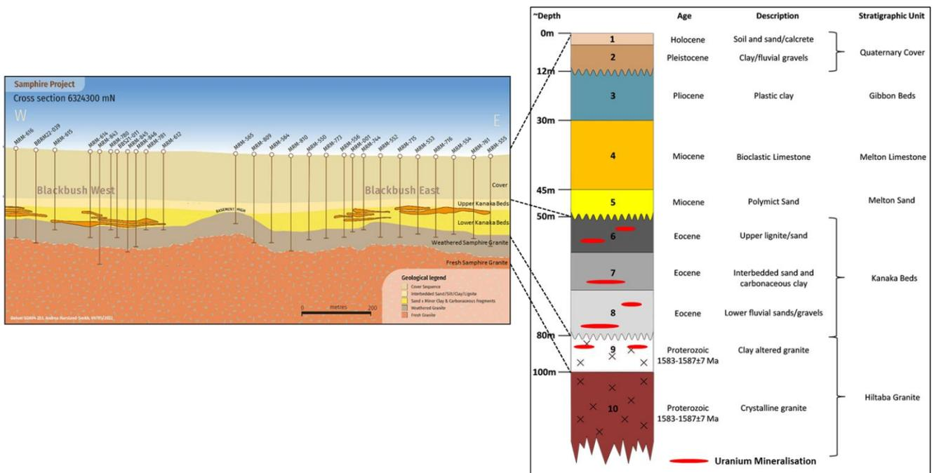
**Figure 3:** Cross section 6324300 mN through the Blackbush Deposit (15x vertical exaggeration, depth in RL metres) showing multi-level zones on simplified geology. Cross section constructed from pU308 intersections from AGE sonic core hole BBRM22-034<sup>9</sup> and historic drilling eU<sub>3</sub>O<sub>8</sub> intersections<sup>10</sup>. Detailed stratigraphic section (modified after USA Internal Report, 2012).
