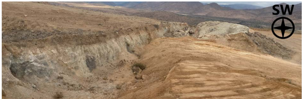
Figure 4-4. Southwest view to the trench ZM-S2. Segment with intense argillic alteration and low Fe grade and low magnetism.
