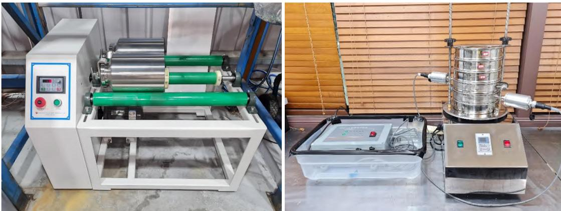
**Figure 1: Ball mill (left) and ultrasonic vibrating screen (right), which enable ALCORE to prepare bath with a narrower range of particle sizes.**
