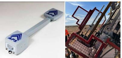
Figure 4: Rig and mast alignment via a Multi-wave Sensors GPS Azimuth Pointing System and a PMD Directa Hybrid north-seeking gyroscope.
