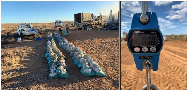
Figure 8: RC samples laid out in rows of 30 x 1m sample piles (1 pile = primary, secondary & bulk samples). Note the weighing rig in use near the end of the second row of samples. At right: Wedderburn digital scale used on weighing rig.
