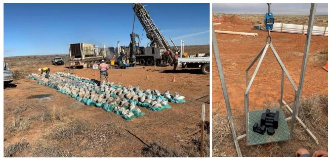
*Figure 9: Magnetic susceptibility measurements being taken on completion of sampling. Samples laid out in rows of 30 x 1m samples. At right: weighing rig being calibrated against the full suite of standard weights (37kg).*
