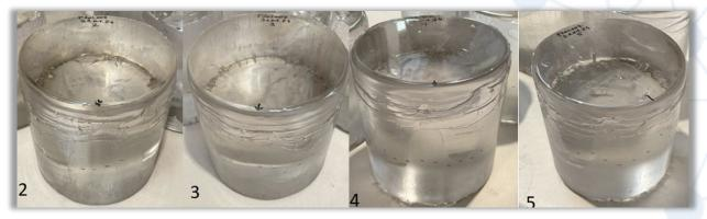
High quality sapphire boules from most recent multiple boule growth using Alpha HPA feedstock material
