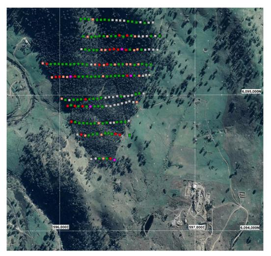
**Figure 2 –** Results of soil sampling program immediately to the north of the Currajong deposit and to the north-west of Adelong Mill
