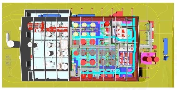
Figure 2: Engineer's 3Dmodel of the designed Lance CPP expansion. The left-hand side 1/3 of the image is the currently existing facility.
