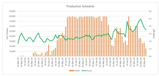
Figure 10: Garden Well Main Production Schedule including Ore Tonnes and Grade
