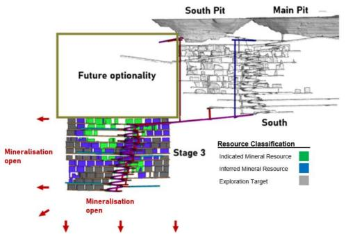
Figure 4: Stage 3 Mine Layout Showing Resource Classifications
