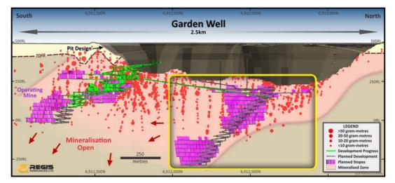
Figure 7: Garden Well Underground Mineral Resource With Drilling, Resource Stope Shapes And Open Pit Design. Garden Well Main Is Highlighted In Yellow And Looking West.
