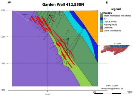
Figure 6: Garden Well Main Cross-Section @ 412,550mN +/- 12.5m
