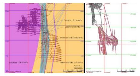
Figure 12: Schematic Rosemont Stage 3 Geology Cross-Section @ 77,350mN +/- 100m
