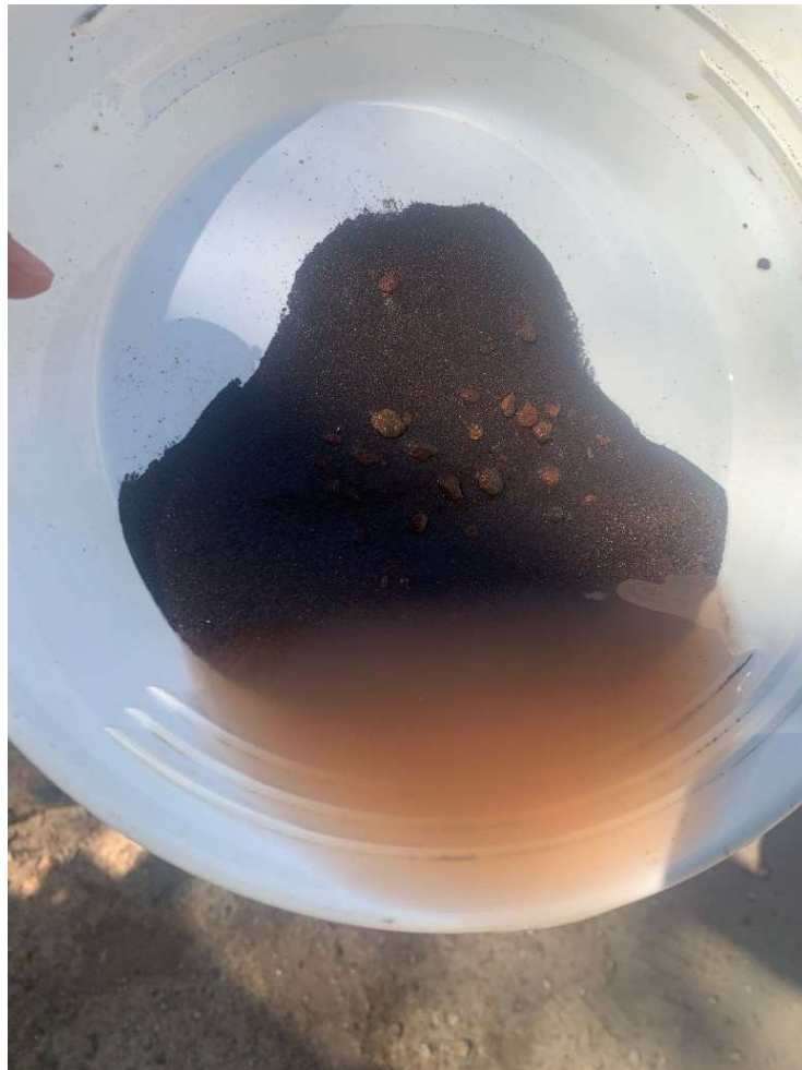
Figure 4 - Panned heavy mineral concentrate from Hole 24WN026 from 7.5 - 9m depth. Interval assay value 53.12% THM
