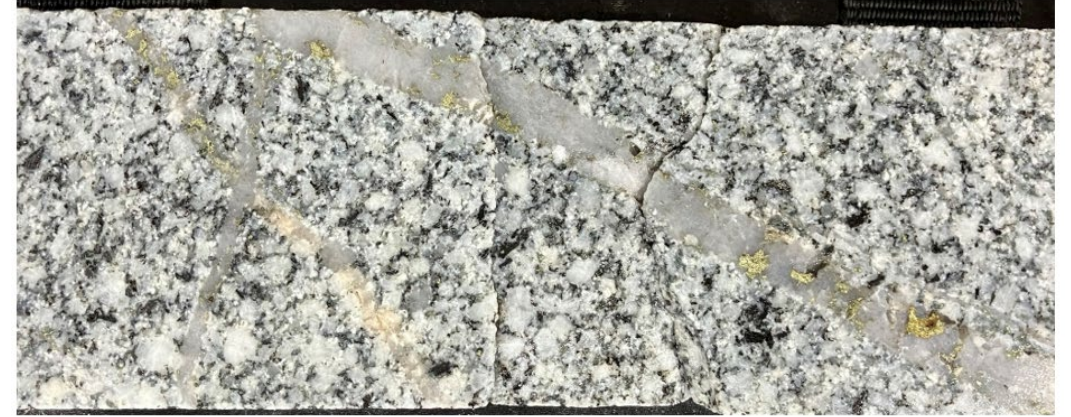
Figure 2. Copper sulphides in mineralised porphyritic granodiorite, Briggs Central. Hole 23BRD0016 at 123.5m. Within a 2m interval of 61mm diameter core which assayed 0.31% Cu.
