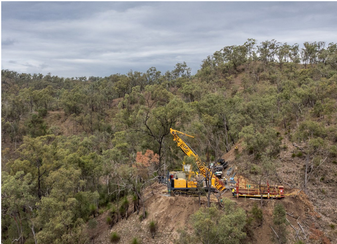
Figure 3. Aerial view of drill hole 24BRD0026. This hole is drilled towards the southwest, across the contact zone between mineralised porphyritic granodiorite and mineralised volcanic sediments in the Briggs Central resource.
