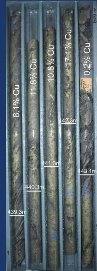
Above & right: Queen Bee drillhole DD24QB0041 from 440.4m to 440.75m, grading in-excess of 10% copper
