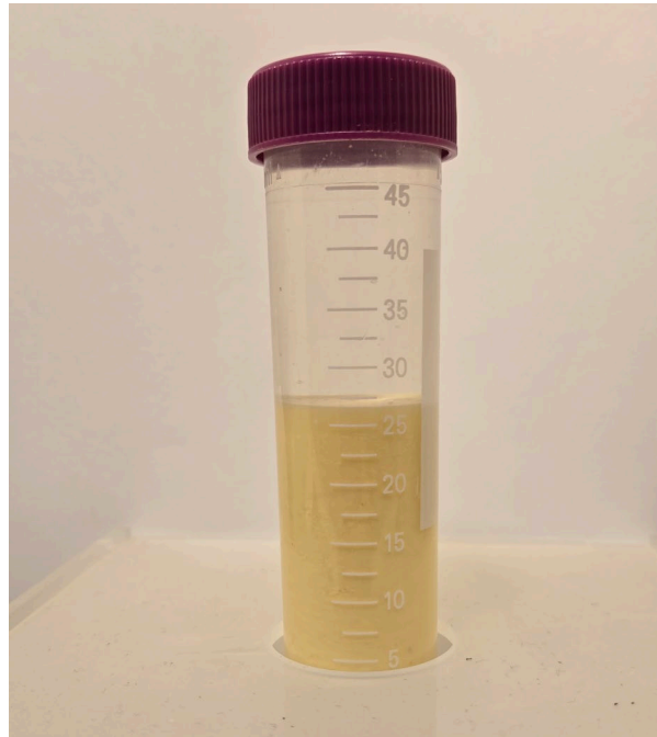
Figure 8: A sample of yellowcake produced from pilot scale process optimization testing at Lance
