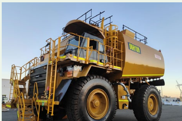
785C water cart after BTP rebuild.
