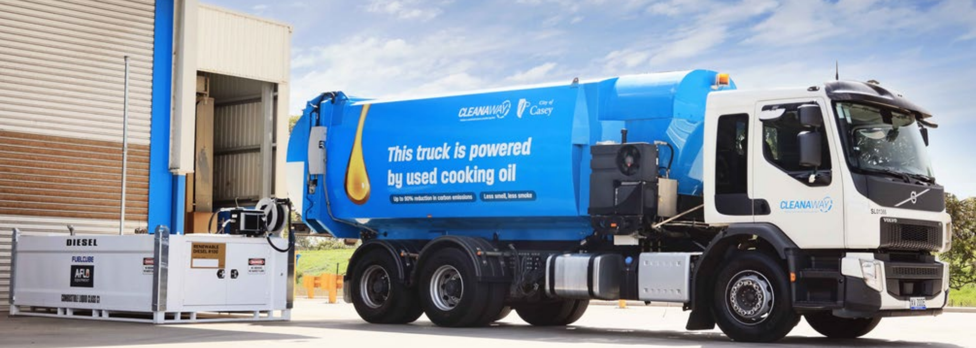
Pictured: Cleanaway/City of Casey side lift truck powered by HVO100
