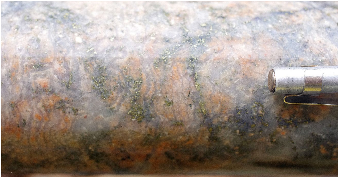
Figure 2. Strongly silicified and altered Briggs granodiorite with micro-UST textures and extensive copper sulphides. Hole 24BRD0026 at 40.5m, from a 2m interval which assayed 1.55% Cu.
