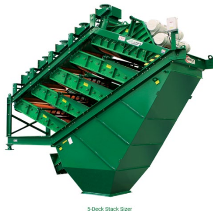
Picture 2: Derrick stack sizer screens
