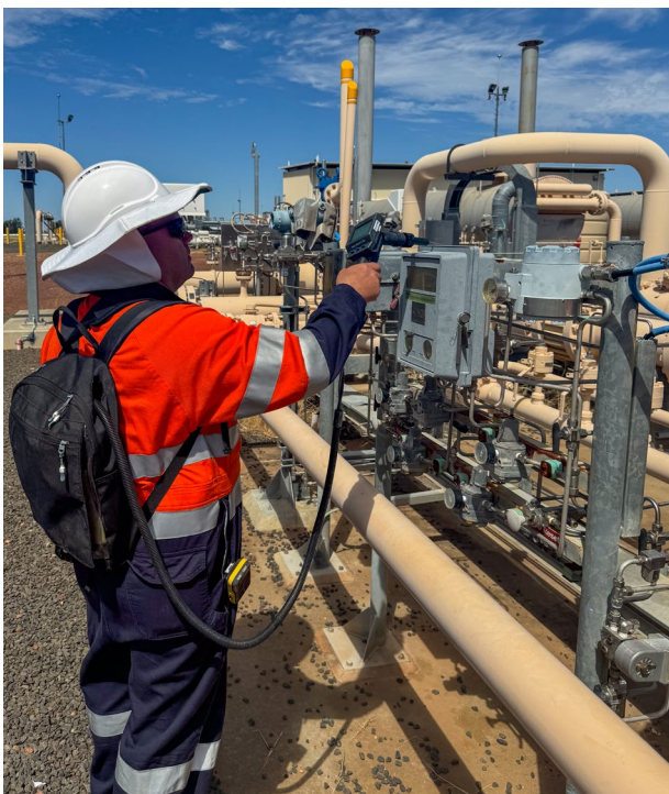
▲ Ground-based, source-level methane measurements during the enhanced methane measurement study at SWQP, QLD
