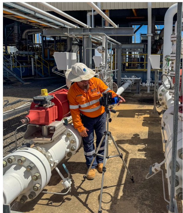
▲ Ground-based, source-level methane measurements during the enhanced methane measurement study at SWQP, QLD
