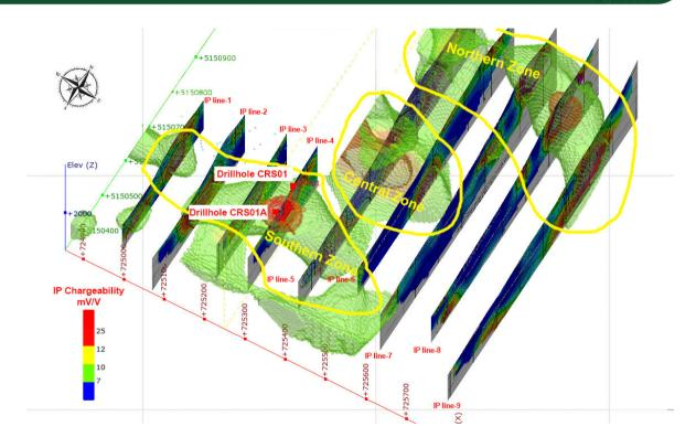
Confirmed encouraging copper mineralisation intersects at Copper Ridge prospect to depth by scout drillhole CRS01A, within continuous anomalous copper for a downhole length of 200.4 m (Assays pending)
