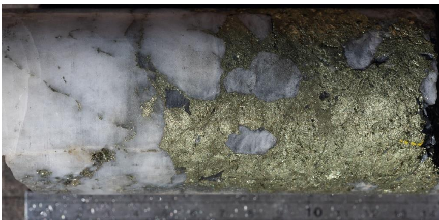
Figure 1 High-grade copper mineralisation in the form of chalcopyrite in magmatic quartz. 24BRD0028 at 39.5m from a sample assaying 2.0% Cu over a 2.3m interval. Core diameter 61.5mm.
