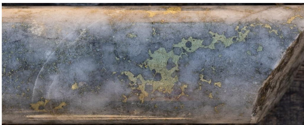
Figure 3 High-grade copper mineralisation in the form of chalcopyrite veins and disseminations in magmatic quartz. 24BRD0028 at 43.3m depth from a sample which assayed 1.83% Cu over a 2.0m interval. Core diameter 61.5mm.
