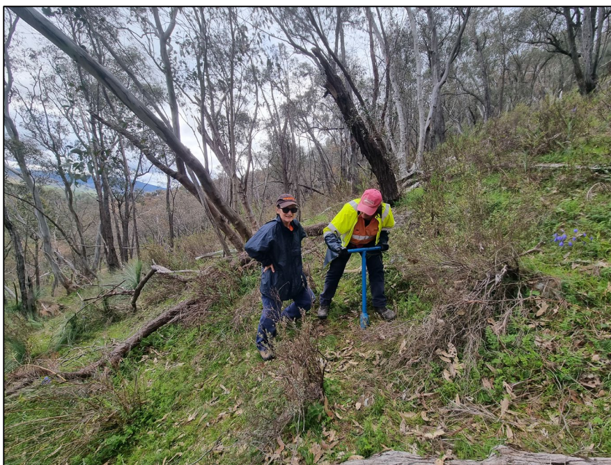
Figure 3 – Augering sample CM24-13 which contained 3.03 g/t gold. The soil sample was collected at 0.15cm depth.
