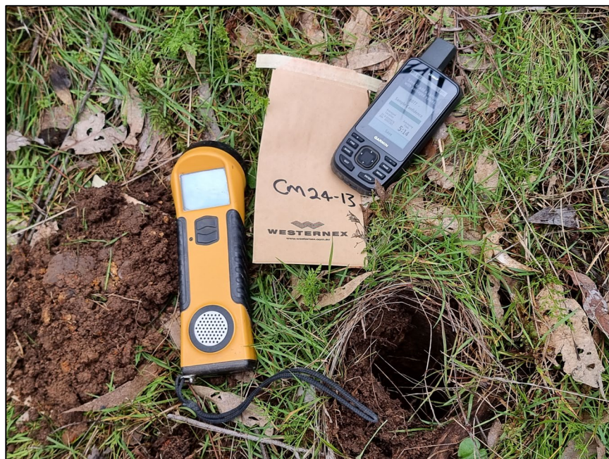
Figure 4 – Sample CM24-13, which contained 3.03 g/t gold. The brown silty clay soil is sitting on kraft paper and has just been measured with the magnetic susceptibility (yellow instrument). The auger hole is backfilled and sealed following the bagging of the sample.
