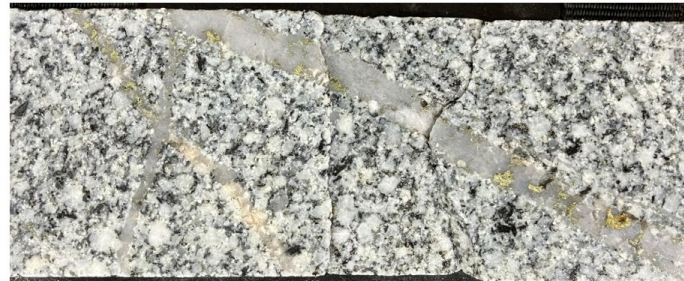
Figure 2. Copper sulphides in mineralised porphyritic granodiorite, Briggs Central. Hole 23BRD0016 at 123.5m. Within a 2m interval of 61mm diameter core which assayed 0.31% Cu.
