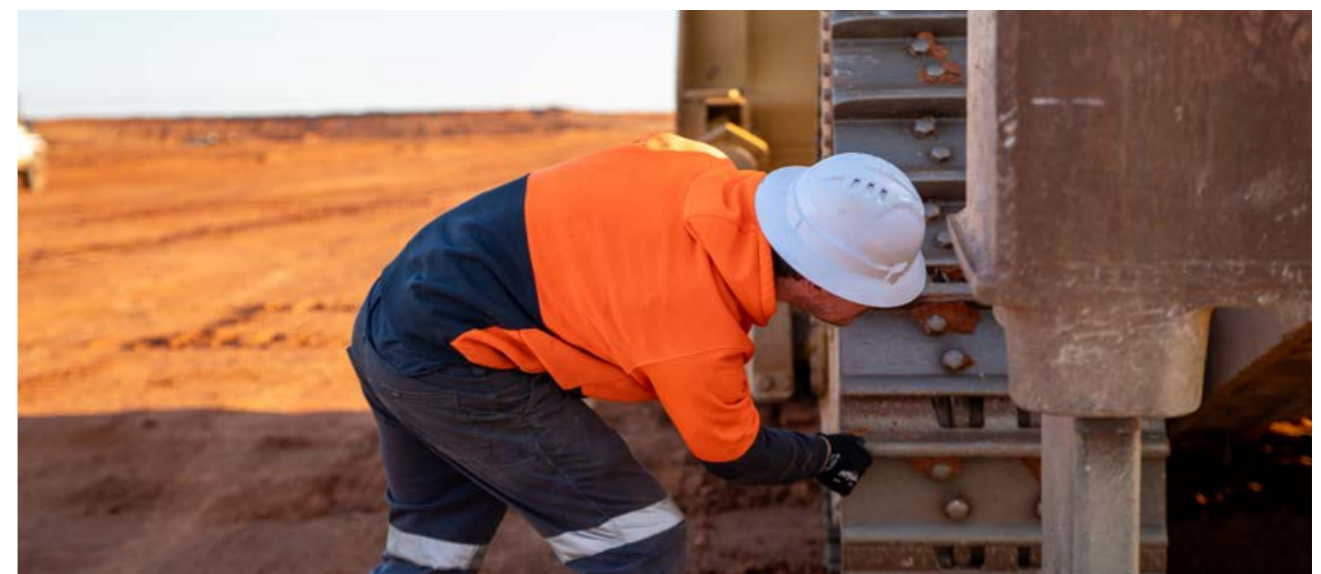
Pre-start checks of a D-9 dozer.
