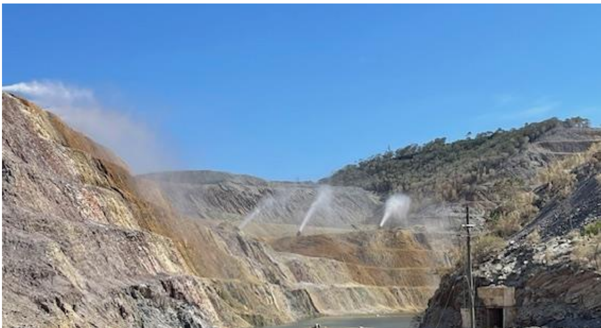
Figure 10: Mechanical evaporators at Esperanza Pit ('EPit')
