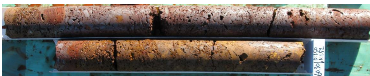
Figure 4: Drill hole METDD029 from 58.8m to 60.3m showing typical canga above Fe enriched hardcap within the Dales Gorge Member
