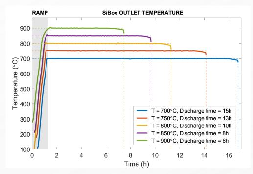
**Outlet air temperature to the process.** Shows 5 runs at various outlet temperature setpoints 医吗
