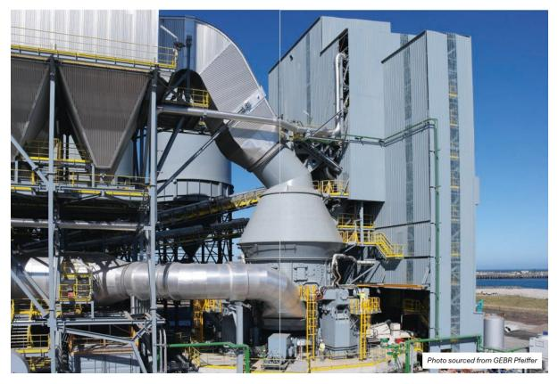
GEBR Pfieffer's MVR 6000 C-6: the biggest vertical mill in Australia operating since 2014
