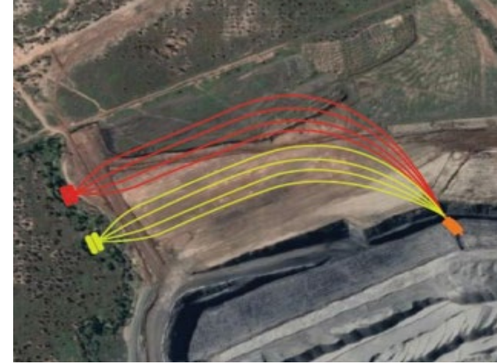
Horizontal drilling concept proposed at the Bengalla Mine.
