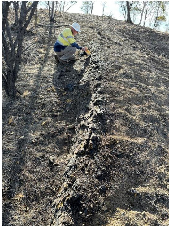
Figure 5. Base Metal Target - Outcropping fine-grained sedimentary rock of the Ronlow Beds with cleavage steeply dipping toward NE - strike NW-SE - yellow-ochre, black & brown limonite possibly derived oxidation of sulphides at depth
