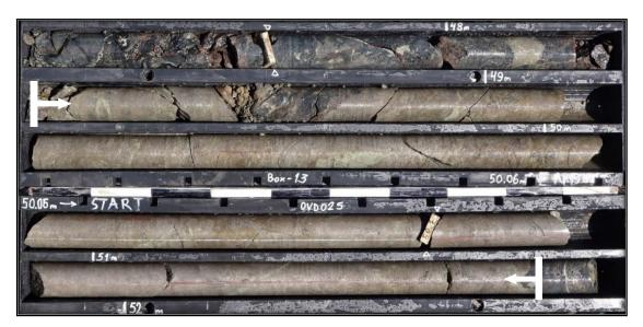
Photo 2. The massive sulphide intersection in the drillhole OVD0254
