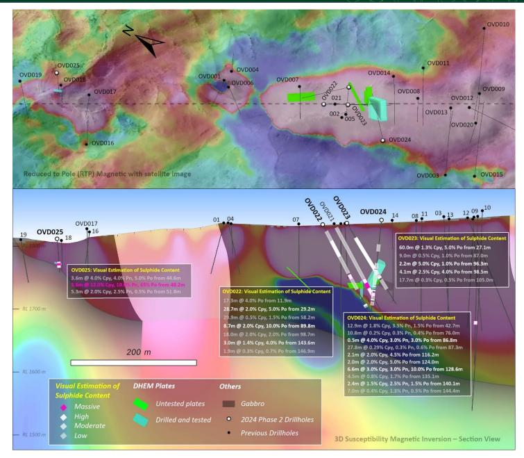
Figure 3. The longitude section of all conductive plates identified by DHEM<sup>8</sup>
