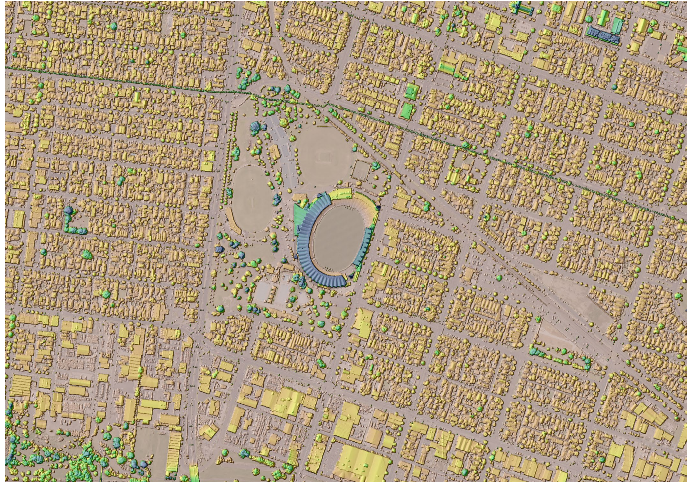
Image: LiDAR derived digital height model of GMHBA Stadium, South Geelong, Victoria
