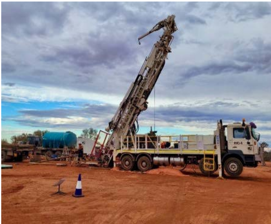
Image 1: Diamond drilling rig testing extensions to high-grade gold mineralisation at Minos
