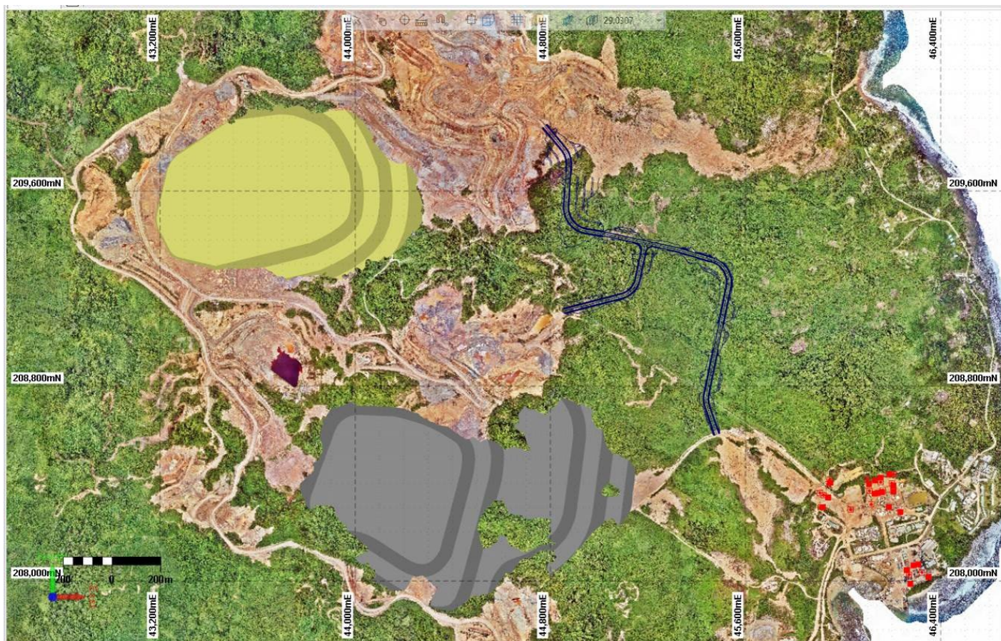
Figure 1. Simberi Sulphides Geotechnical Drilling Campaign (comprising Middle and Darum waste rock dumps; new ball mill location; new ROM pad; new haul road and wharf / concentrate shed areas)
